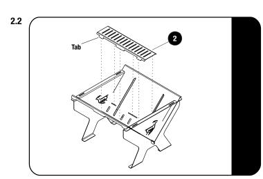
Place the Burner Plate (Item 2) inside the assembly.
